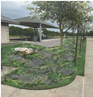
ADD NEW TYKE TRACK AROUND PLAYGROUND & NEW PLANTING BEDS WITH SHADE TREES. VERIFY UNDERGROUND UTILITIES. TREES TO BE PLANTED A MIN. OF 5' FEET AWAY FROM UTILITY LINES.
