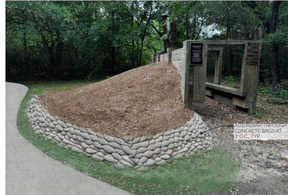
LOW EROSION WALL AT OVER THE TOP MONUMENT TO PREVENT HILL FROM SLOUGHING ONTO SIDEWALK. CREATE RETAINING WALL AT TOE OF HILL USING BAGS OF CONCRETE, WETTED AND STACKED IN LIFTS UP TO FOUR BAGS HIGH. BAGS TO BE BURNED OFF AFTER CONCRETE HAS CURED. INCORPORATE REBAR THROUGH BAGS.
