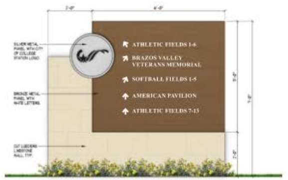
① ROUNDABOUT WAYFINDING SIGNS (EXAMPLE) REF. SHEET 4 FOR SIGN LOCATIONS UNDER ROUNDABOUT IMPROVEMENTS SCALE: 1" = 1'-0"
